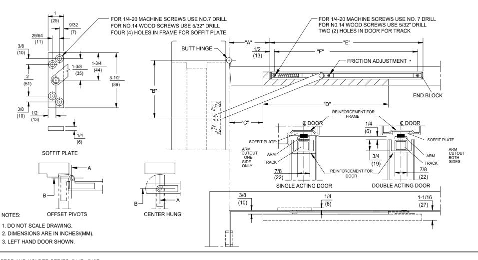
STOP AND HOLDER SERIES: 711F - 713F STANDARD DUTY CONCEALED FRICTION/STOP SINGLE ACTING AND DOUBLE ACTING DOORS CENTER HUNG. 3/4" OFFSET AND 4-1/2" X 4-1/2" HINGES
